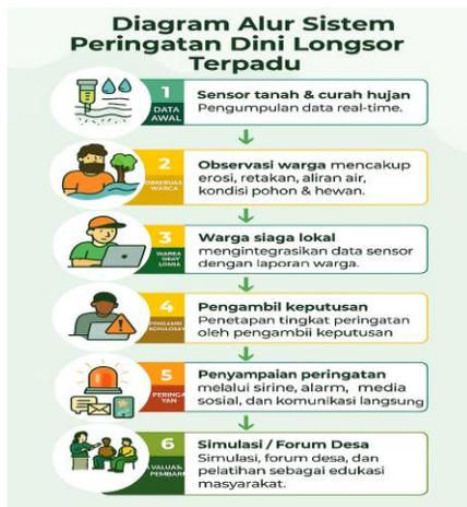
Gambar 2.3. Diagram Alur Sistem Peringatan Dini Longsor Terpadu
